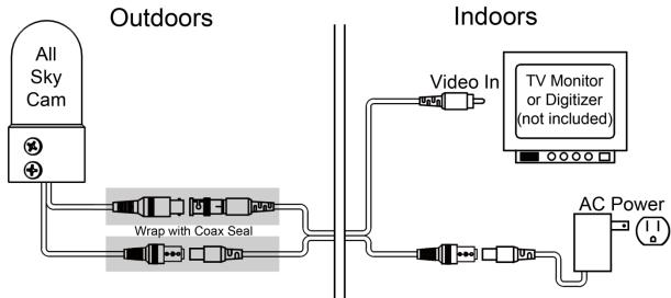
After establishing a mounting for the camera, pass the camera's wires through the pole (if applic able) and connect it to the supplied extension cable. Then cable connections must then be wrapped with the included Coax-Seal weather stripping to prevent rain or dew from shorting out the power and video signals. See the Coax-Seal envelope for instructions. The extension cable can then be routed through the pole and into the building inside.
